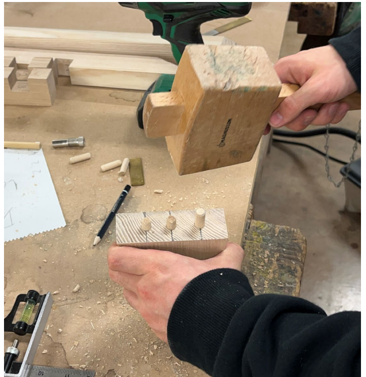
Marking and drilling holes for the dowel pins to use in attaching the feet to the base frame
