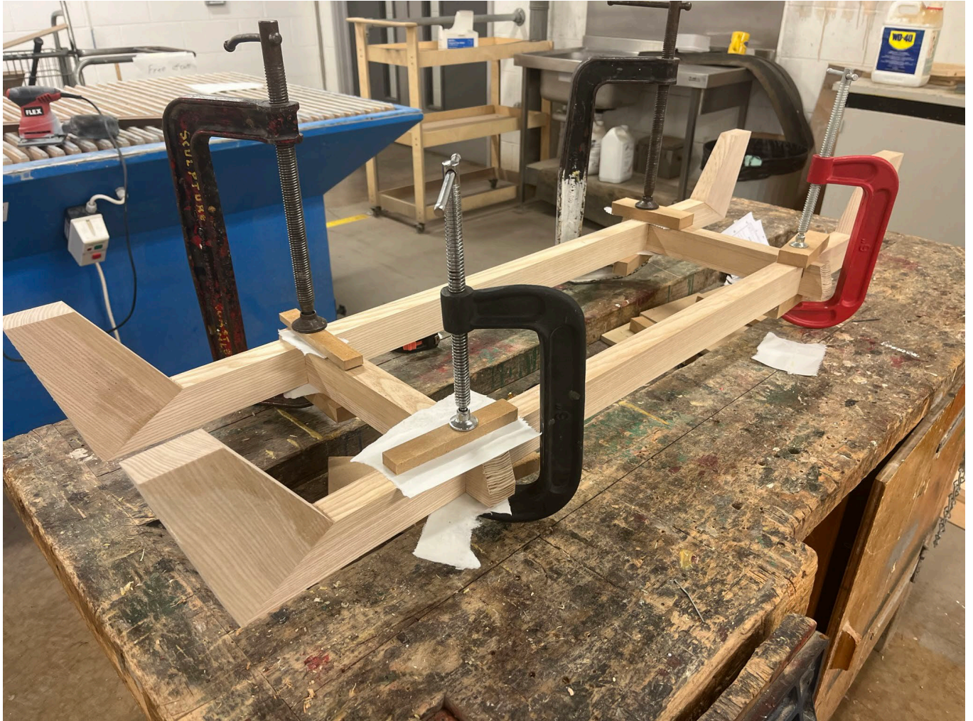
Gluing the frame together
