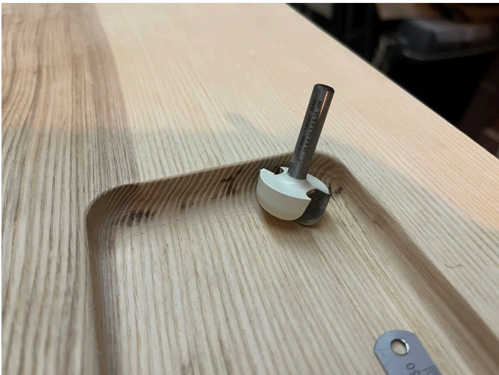
Dish-shaped routed-out drawer recess
