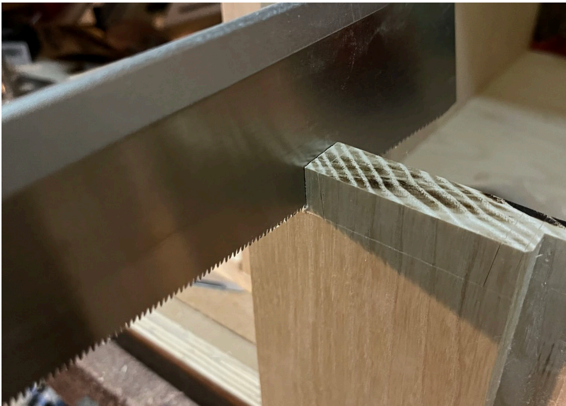
Dovetail joint marking and cutting
