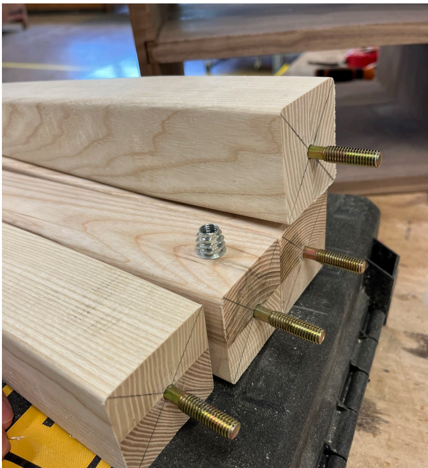
Drilling holes and fitting threaded bolts
