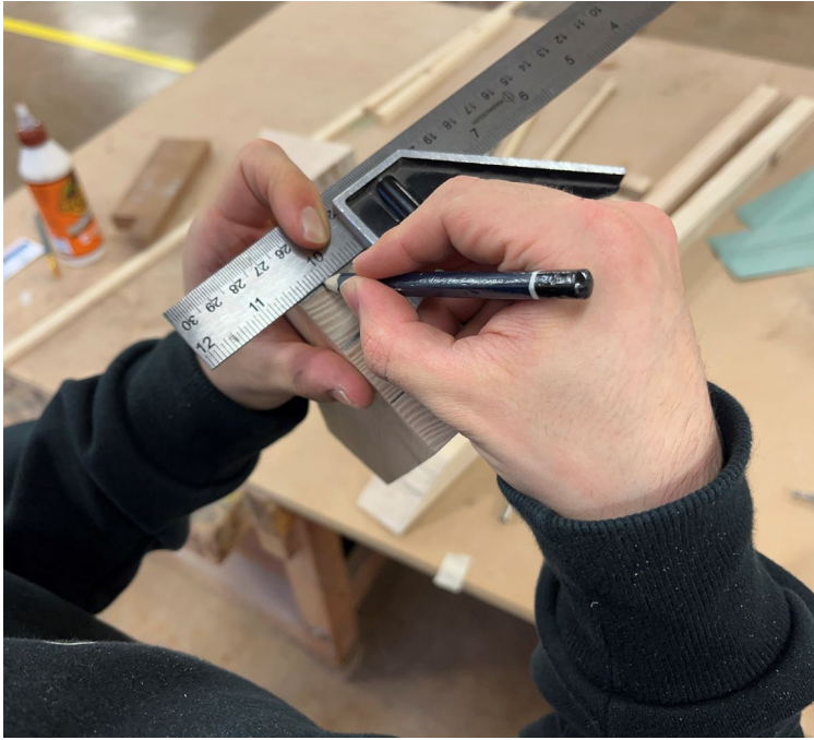
Marking and drilling holes for the dowel pins to use in attaching the feet to the base frame
