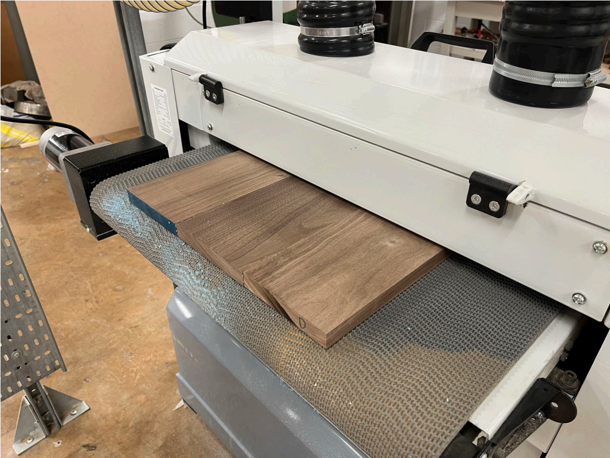
Drum sanding flat and gluing up
