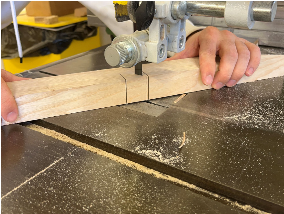
Cutting out the half-lap joints
