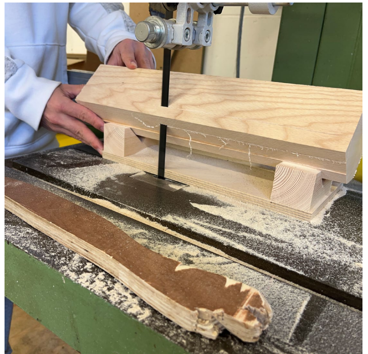
Trimming corners off with self-made jig
