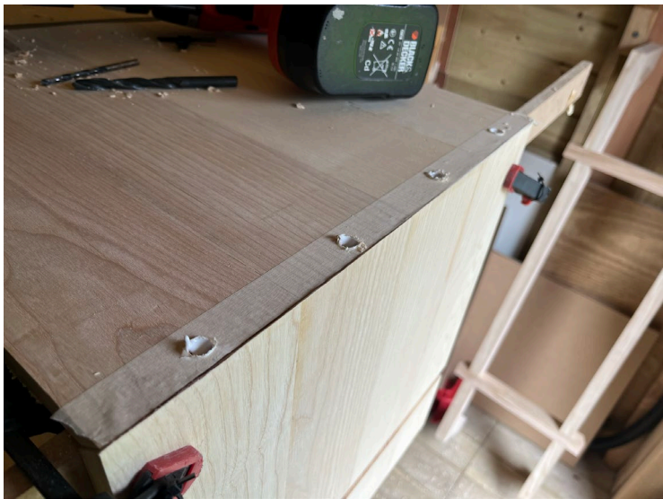
Dowel drilling and pinning for mitre joints
