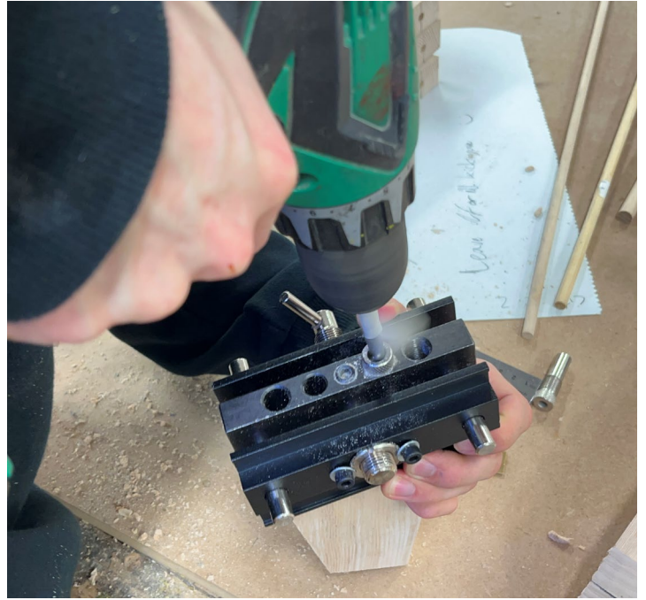
Marking and drilling holes for the dowel pins to use in attaching the feet to the base frame
