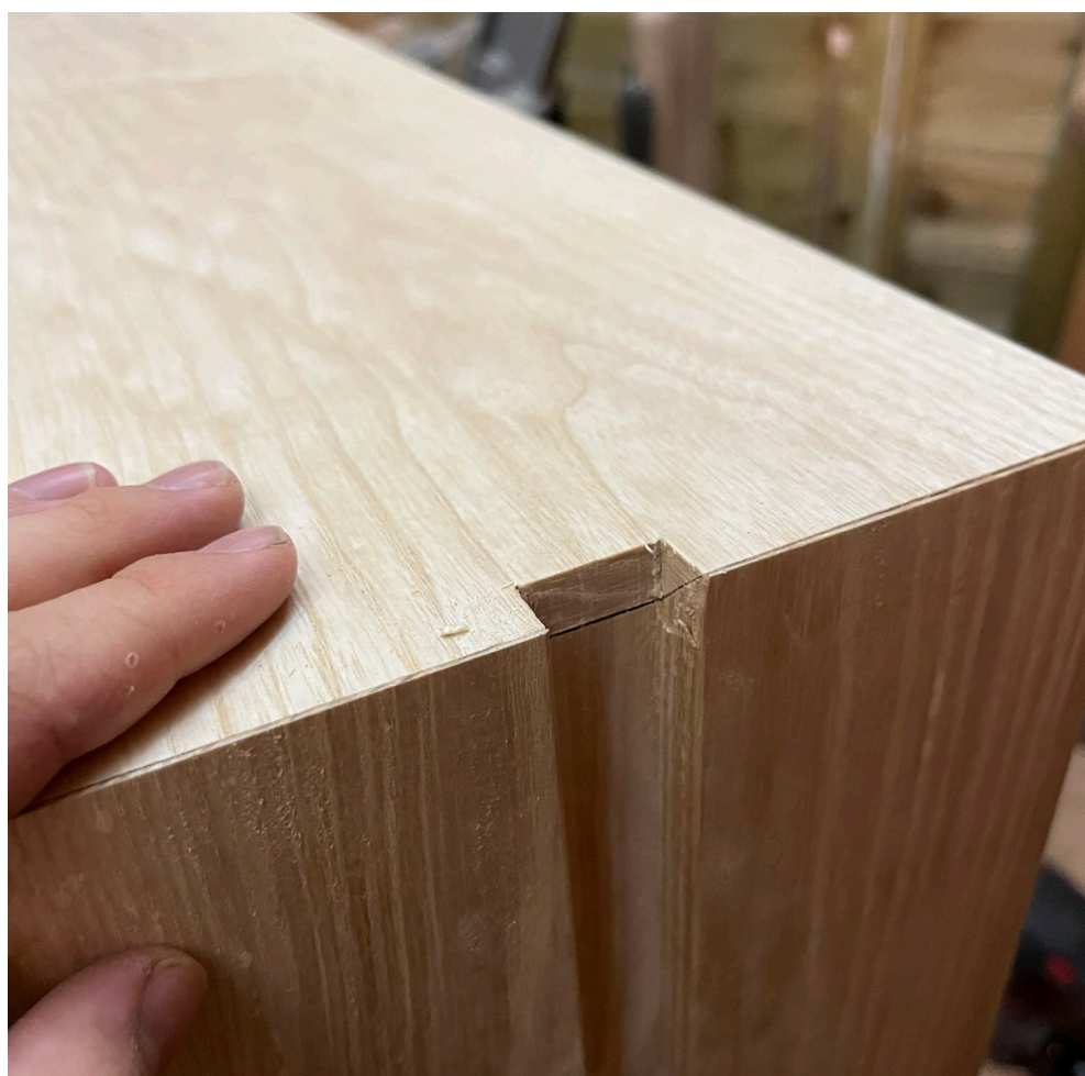
Mitre joint for drawer back and slot cut for drawer runners
