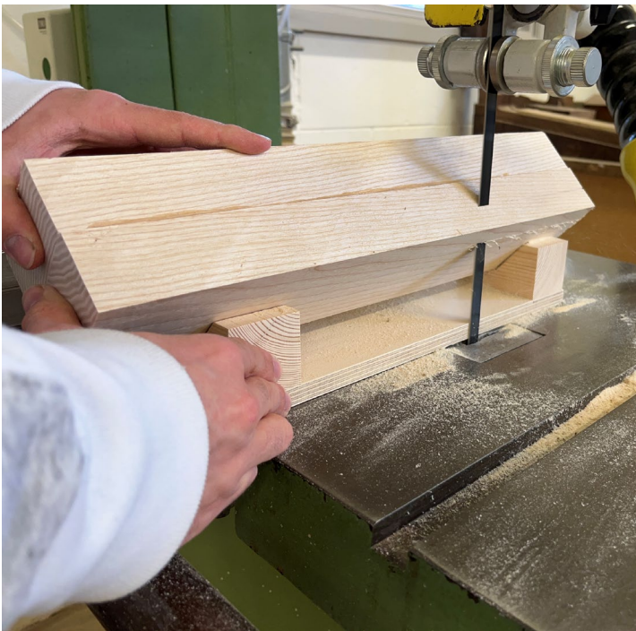
Trimming corners off with self-made jig
