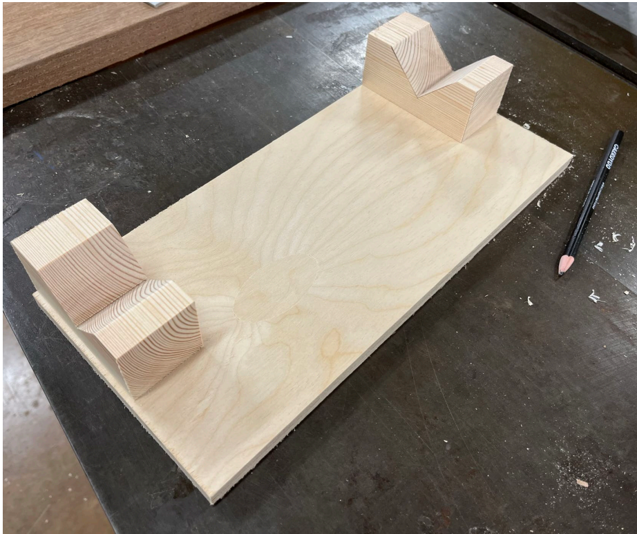
Trimming corners off with self-made jig
