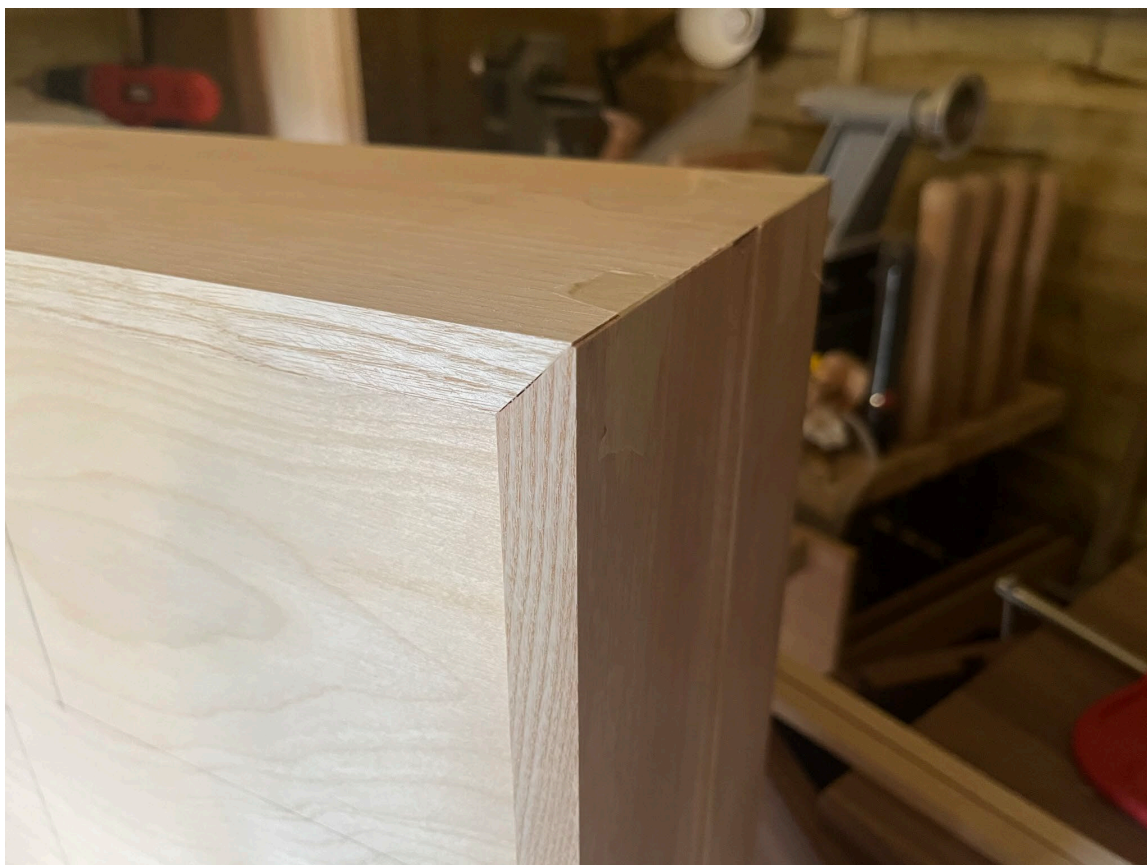
Mitre joint for drawer back and slot cut for drawer runners
